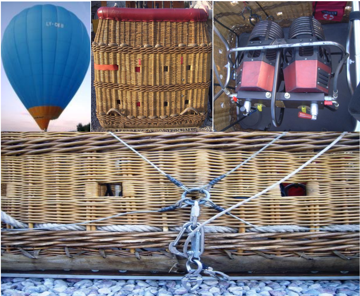
LY-OEB Schroeder Fire Balloons G 30/24. Built 2000. Schroeder V basket. Schroeder FB5 burner. 4x Worthington tank.
